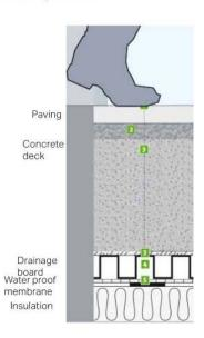
Figure 12. Intensive Green Roof: Substrate and Structure
