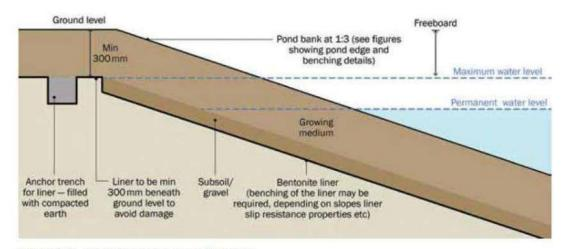
Figure 23.13 Details for a typical geosynthetic liner
