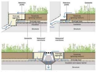
Drainage systems for an extensive green roof.
